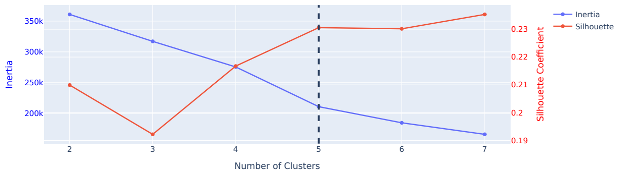
Figure 7: Inertia and Silhouette plot of different cluster sizes. As one can see, the inertia has an "elbow" at a cluster size of five. Similar, the silhouette shows one of its highest values at a size of five as well. Thus, we select a cluster size of five.
